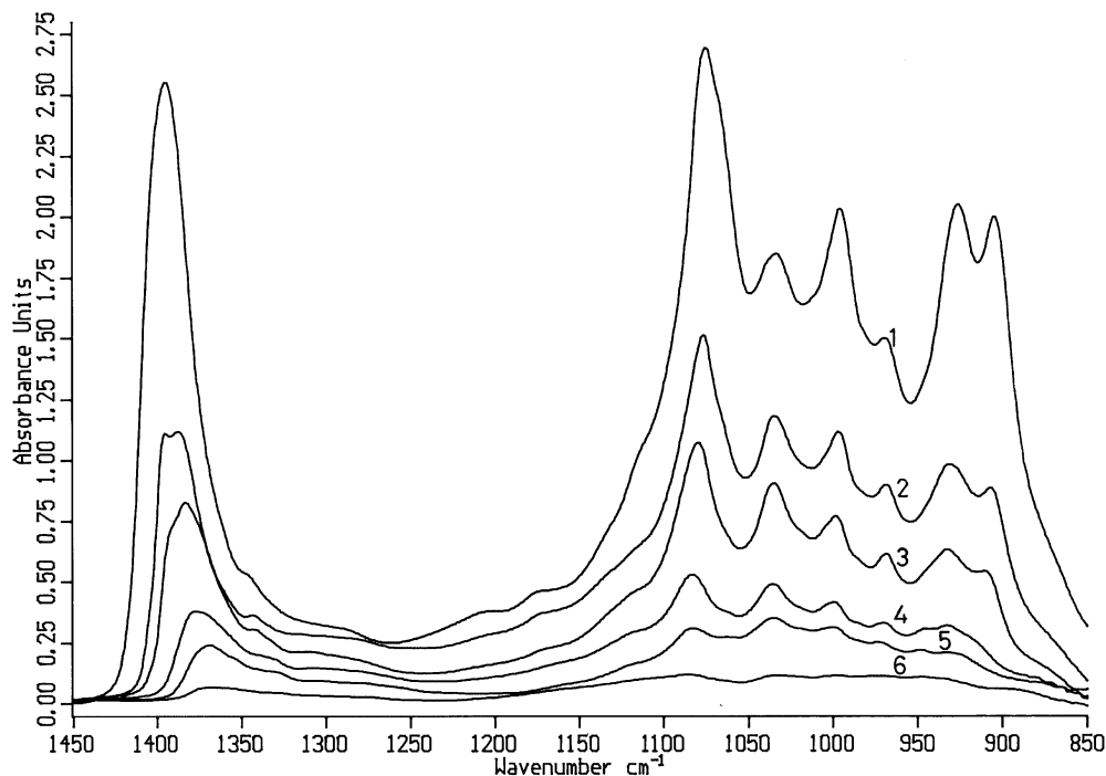
FIG. 1. Infrared spectra (sulfate region) of the different samples studied: 1 , SZ873; 2 , SZ1073; 6 , SZ1173; 3 , 4 , 5 , see text.
